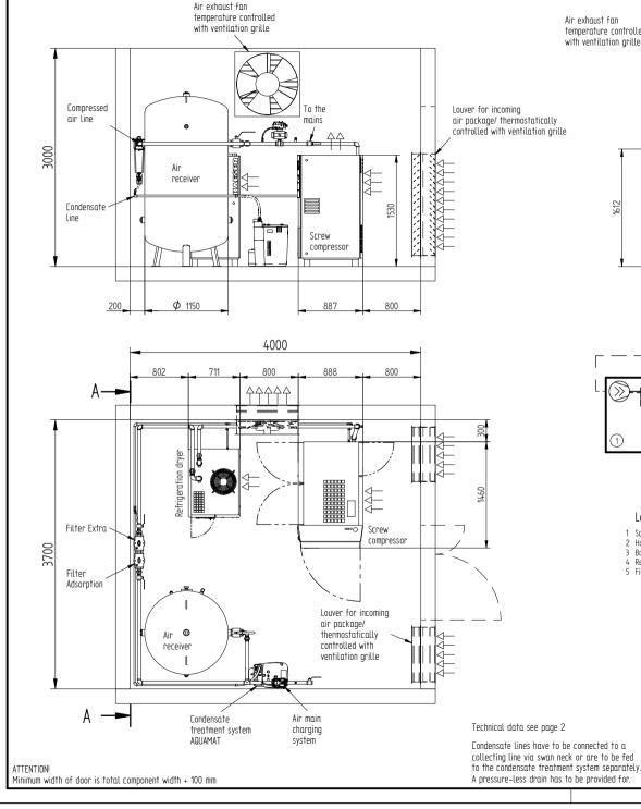
Design limits for ambient temperature + 3° [ тпх: + 40° [
