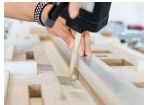
...or applying multi-component adhesive.
